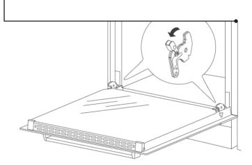
**REMOVAL OF THE INTERNAL GLASS PANEL** Unscrew and unfasten the plastic latch that is in the corner at the top of the door. Next take out the glass from the second blocking mechanism and remove. After cleaning, insert and block the glass panel, and screw in the blocking mechanism.
