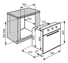
Note. It is a requirement for a ventillation gap to be cut into the oven cabinet as per the diagrams on this page.
