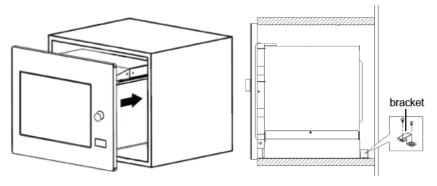
4. FIX THE MICROWAVE IN TO PLACE - Open the door and fix the microwave into place using Screw B, through the installation hole (indicated in the diagram below). Then fix the trim-kit to cover the installation hole.
